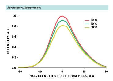
Test Conditions: I (Pulsed Mode) = 100 mA
