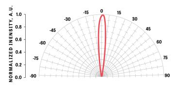
Test Conditions: I (CW) = 100 mA, CW=Continuous Wave Mode
