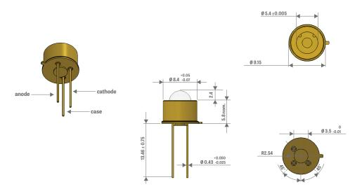
All dimensions are in millimeters. Unless noted otherwise, all dimensions have a tolerance of  $\pm$  0.05 mm.
