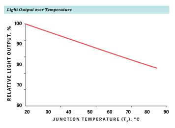
Test Conditions: I (Pulsed Mode) = 100 mA
