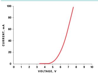
Test Conditions: I (Pulsed model)=1 to 100 mA; Case Temperature ( $T_c$ )=25°C
