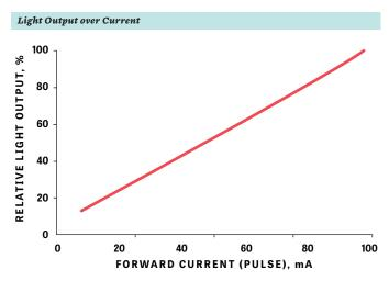
Test Conditions: Case Temperature ( $T_c$ ) = 25 °C
