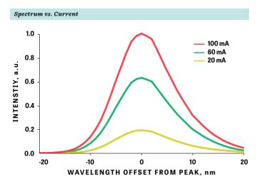
Test Conditions: Case Temperature (T<sub>c</sub>) = 25 °C
