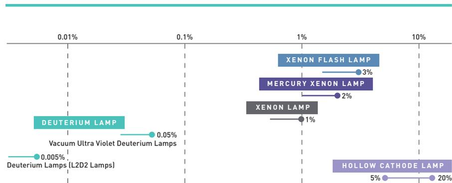
Stability of light output for various traditional UV light sources. Source: Adapted from Hamamatsu Light Source, [http://www.hamamatsu.com/resources/pdf/etd/LIGHT\\_SOURCE\\_TLSZ0001E01.pdf](http://www.hamamatsu.com/resources/pdf/etd/LIGHT_SOURCE_TLSZ0001E01.pdf), Apr. 2014.]
