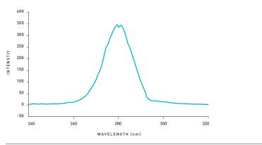
Effective germicidal power plot obtained after convolution.
