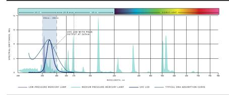
Comparison of emission spectrum of low-pressure mercury lamp, medium pressure mercury lamp, UVC LED and typical DNA absorption curve. The curve depicted for the UVC LED represents a typical commercial UVC LED for disinfection applications.
