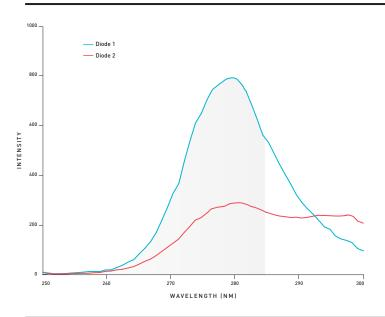
Spectra of two diodes and gray area showing the area of germicidal activity. The UVC LED spectrum for Diode 2 shown is an extremely imperfect emission example for demonstration purposes—not characteristic to commercially available UVC LEDs.
