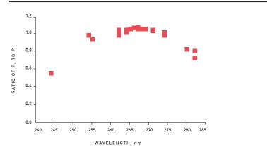
Shows the effect of wavelength on the power output ratio of  $P_0$  to  $P_t$ .
